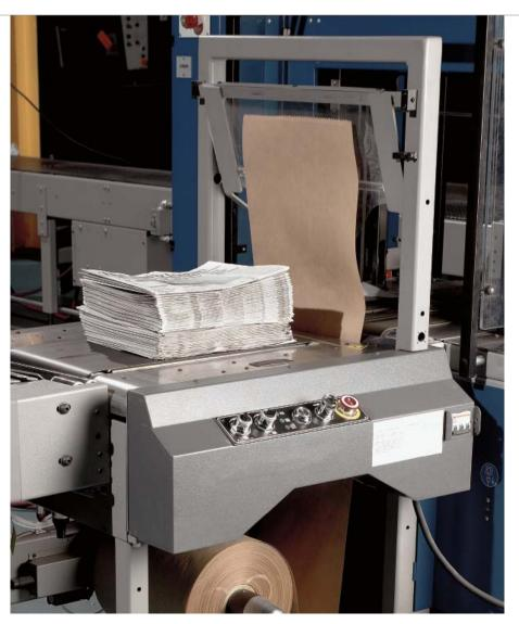
The Goss® Eclipse® Bottomwrapper quickly and efficiently applies protective kraft paper to the bottom or to three sides (optional). It handles a wide variety of bundle shapes and sizes and is designed for close-coupled stacker operation or down-stream placement in tie lines. The unit is equipped with a proprietary paper feed system. High bundle throughput helps reduce bottlenecks at the delivery end of the packaging center.
